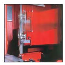
The guide arm automatically adjusts to maintain the maximum beam strength of the blade throughout the cut.
