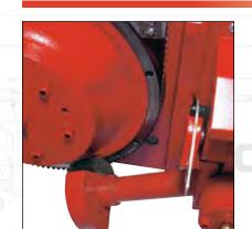
The wire brush automatically adjusts for maximum efficiency and eliminates excessive brush wear.
