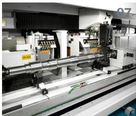
**01** External grinding of extrusion screw | **02** External grinding of turbine propeller | **03** Face grinding of wind energy shaft | **04** External grinding of spindle | **05** External grinding and measuring of transmission shaft | **06** External grinding and measuring of printing roll | **07** Grinding of railway shaft in a grinder with double grinding wheelhead
