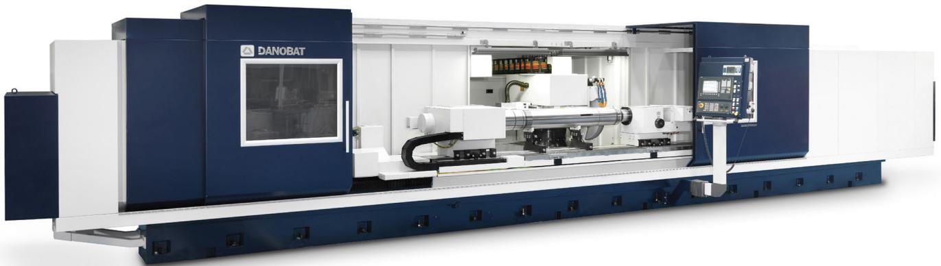
**This moving table grinding machine range has been designed to fulfil the requirements of a wide range of applications that combine external, internal, face and taper grinding of components such as: transmission shafts, electric motor shafts, gas and wind turbine shafts, railway shafts, machine tools shafts, landing gear components, etc. Depending on the application corundum, CBN or diamond wheels can be used.**
