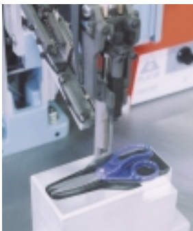
Model SD-110 Screwdriver with optional Magnetic Particle Clutch mounted on a Base with customized fixture.
