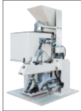
Model SD-122-1 Screw/Nut Driver with Sound Enclosure over Feeder and Supply Hopper
