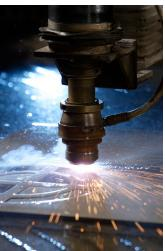
ESAB's exclusive patent allows you to combine the non-thermal waterjet process with the thermal plasma cutting process on the same gantry. The Hydrocut LX can be equipped with ESAB's m3 Plasma systems from 200 up to 720 Amps. The air-curtain option allows the plasma to cut underwater, as well as the water jet. Fast switching and automatic process control allows both plasma and waterjet tools to be used on the same part.
