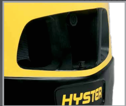
Counterweight tunnel design improves airflow
