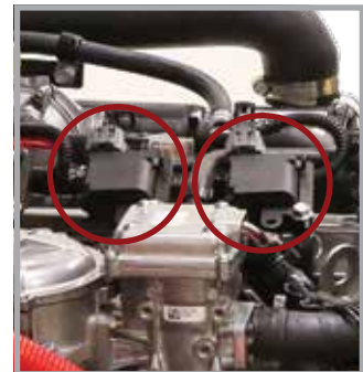
Coil over plug ignition design
