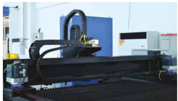
The low weight aluminum undercarriage ensures high dynamic precision.
