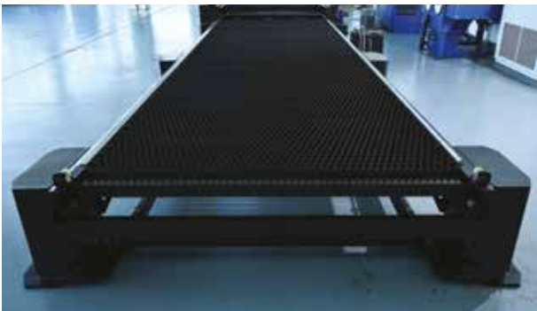
Automatic pallet changer for continuous operation.
