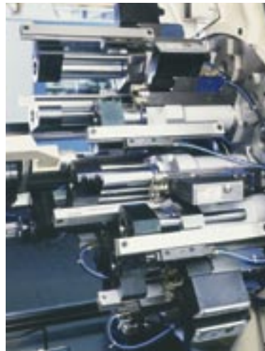
Drive housing with hydraulic endworking slide drives
