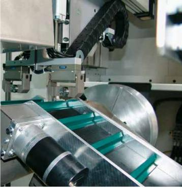
Precision and the visual appearance of the parts being manufactured in today's market are becoming more and more stringent. Dents, marks and flaws are no longer permitted. In order to meet these requirements, Tornos developed a dual parts handling system, which picks up the parts and conveys them directly to the machining area and then conveys them outside of the machining area.
