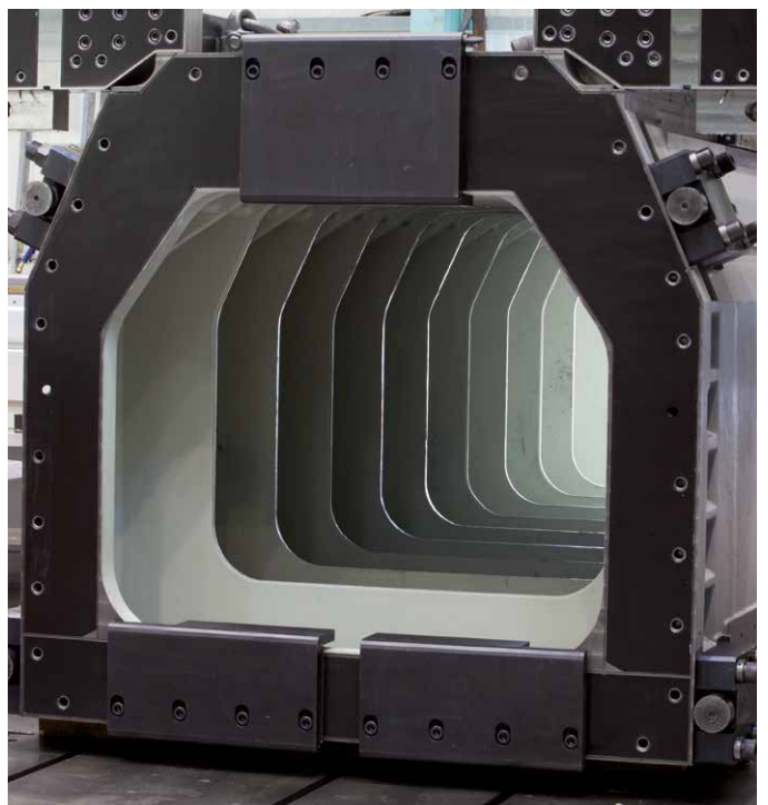
Robust, strongly ribbed machine column
