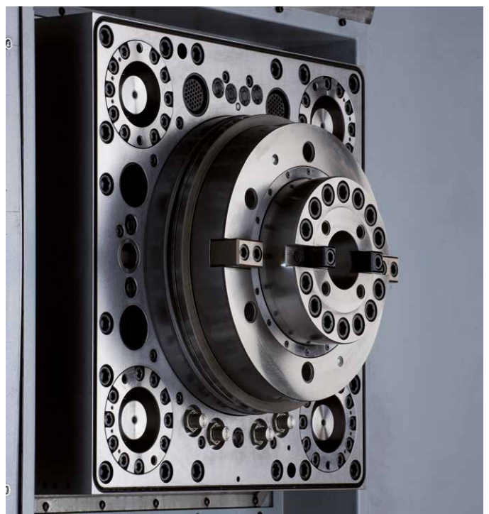
RAM with an automatic adapter plate
