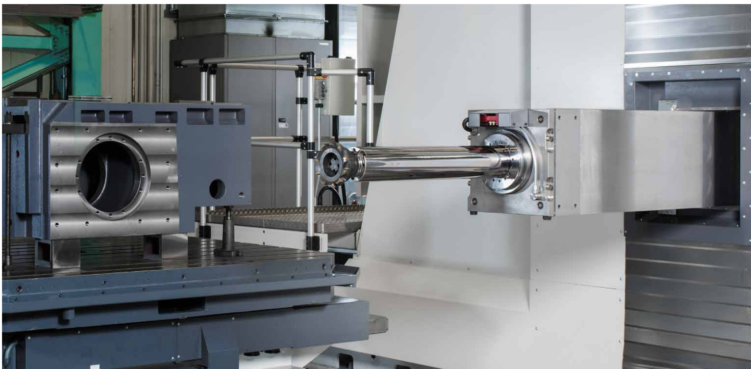
Far extendable RAM and boring spindle
