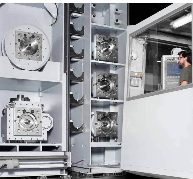
Pick-up station for several milling heads and additional space for special-purpose tools
