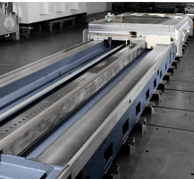
Hydrostatic guides of the robust machine bed
