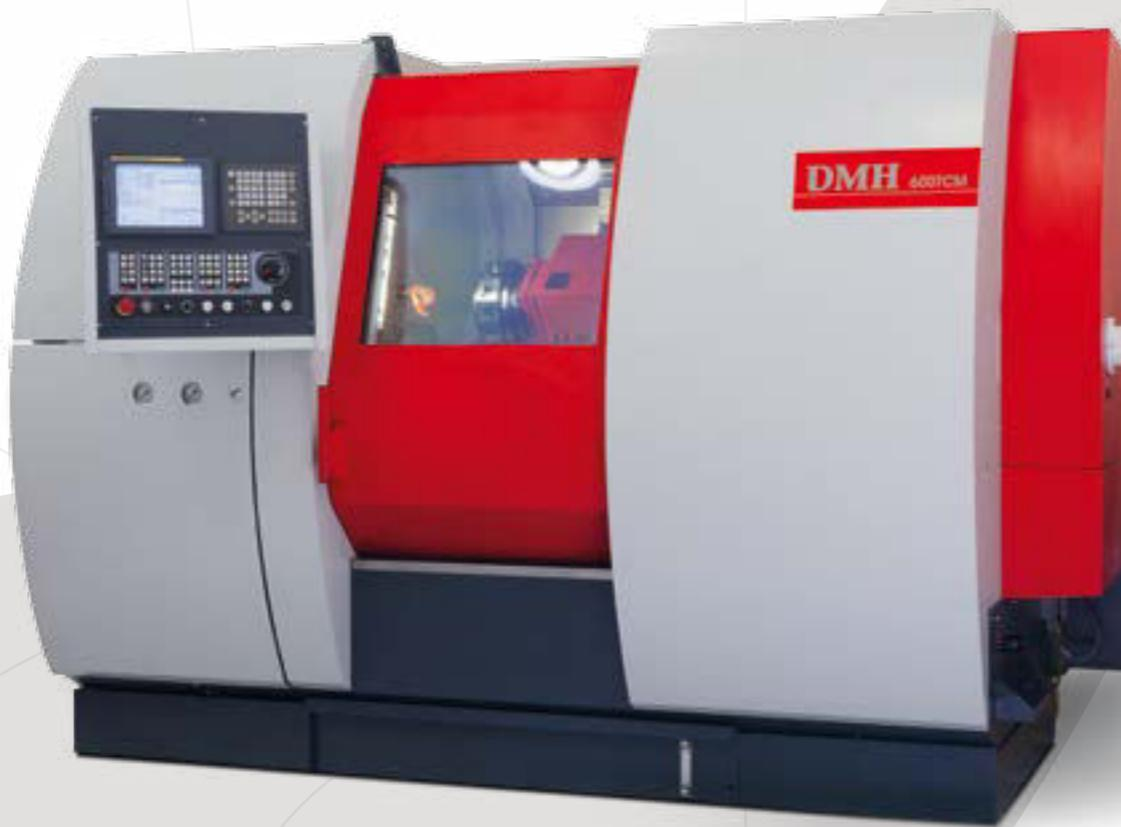
The DMH 600TCM is a versatile competence centre for turning, drilling and milling work within 4 axes. The unconventional design of the machine makes it unique and distinctive. Faster, better, more powerful are all those attributes with which this system can be described at its best. Only those having the most stringent demands should take this machine into consideration.
