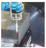
Infrared measuring probe
