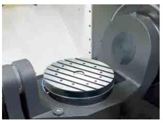
Rotary swiveling table with parallel grooves
