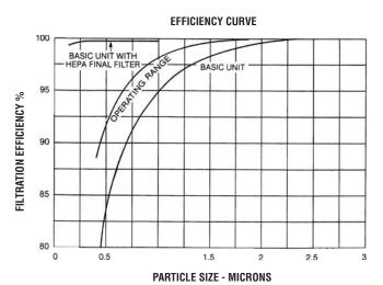
Unit rated in an actual working condition with the filter element saturated with oil. Due to the centrifugal action, the collection media is continuously cleaned and there is no appreciable pressure drop, as in the case of static media type devices.
