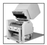
Hydraulic tilt mechanism for the infeed hopper provides complete access to the cutting chamber and rotor.
