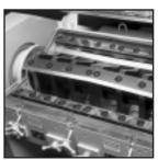
Twinshear™ knife configuration increases cutting efficiency
