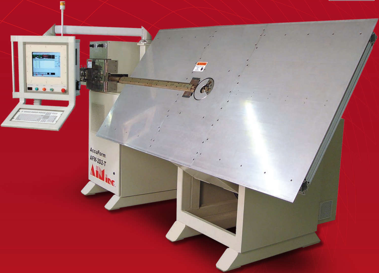
AFM-2D shown without safety barrier for display purposes.
