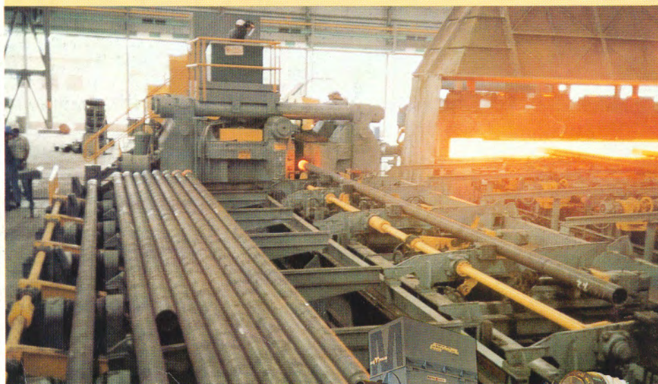
Fully automated tube upsetter installation for tubes 4 inches through 10 3/4 inches in diameter.
