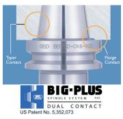
draw bar pulling pressure, moves further into the spindle. On high tolerance applications, this slight pull back of the cutter can affect dimensional accuracy of the Z-axis. Pull back can also cause the toolholder to get locked into the machine spindle taper. The face contact provided by the BIG-PLUS Spindle System prevents the toolholder from being drawn back into the machine spindle.
