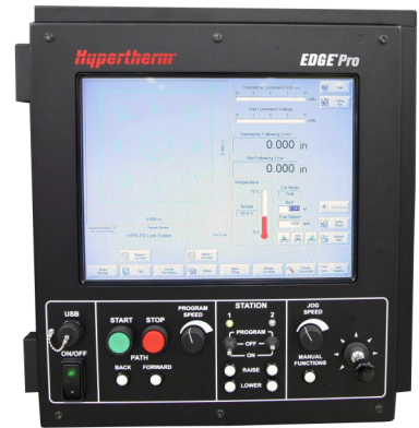
Aviator DSD Equipped with the Hypertherm EDGE-Pro CNC Controller with integrated Height Control System.
