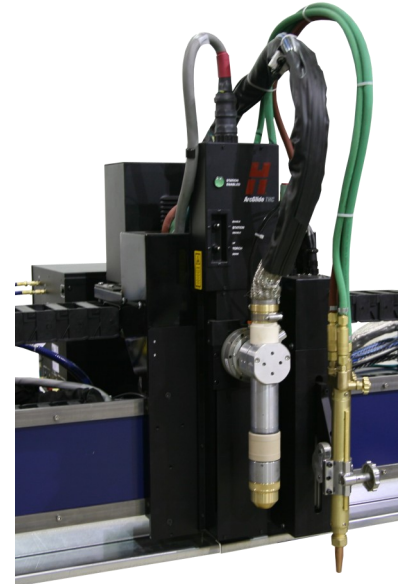
Aviator DXD Master Carriage shown with Hypertherm HPR-260 Plasma Torch, ArcGlide THC Lifter, Collision Sensor, and Oxy-Fuel Torch.
