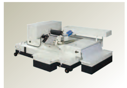
COOLANT SYSTEM WITH AUTO. PAPER FEEDING DEVICE AND MAGNETIC SEPARATOR (WITH 1 ROLL OF PAPER) B17-0302X Volume : 120L Paper feeding motor : 25W Pump : 1/8HP Coolant Capacity : 20L/min. Space :1,450 x 620mm ( 57" x 24 3/8" ) Height : 760mm (30" )
