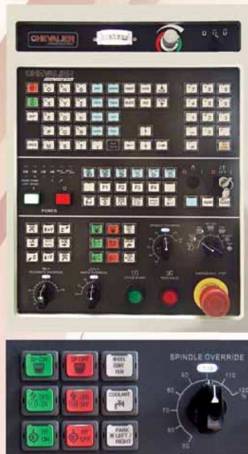
A light has been added to ensure ease of spindle speed monitoring at 100% spindle override position.
