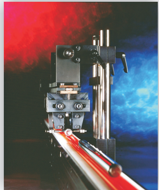
Adjustable-size "rolling V" top guide for various-diameter long rods on TFD-24
