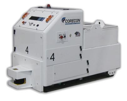
The Eagle E275 AGV is an automated tugger that is designed for applications requiring automatic assembly, or delivery of parts within a manufacturing or production facility. This AGV is ideal for towing single or multiple carts, to pick up and deliver parts to various points within a facility or to integrate with assembly workstations. The Eagle E275 is capable of towing loads of 7,500 lbs with an optional drive assembly that can tow 20,000 lbs.
