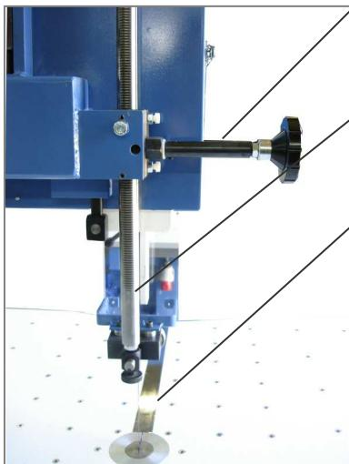
Automatic and perfect adjusting tension of the knife through mechanic wheel.
