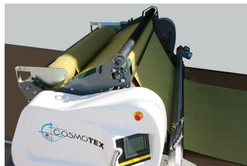
Cradle feed with single piece CONVEYOR BELT.
