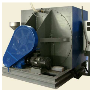
Back view of the machine. Engine power located in accessible place near the floor, for easy maintenance
