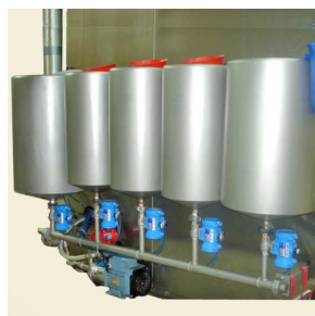
Automatic programmable dispenser by pumps and PLC interface
