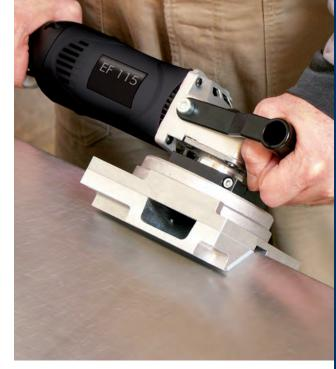
The handy ROLEI® EF 115 can deburr and facet large, heavy parts with ease. The precise edge control guarantees clean bevels at an angle of 45°.
