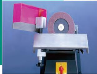
Beveling and deburring machine with a fixed beveling angle of 45° and an infinitely adjustable beveling width from 0" to 3/8" for all metals from stainless steel to aluminum. Precise adjustment of the face width using a hand wheel.
