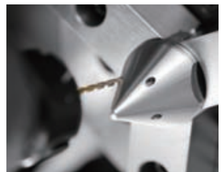
Small hole machining using a universal tool holder
