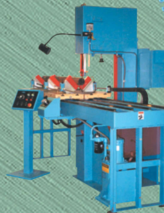
2013-V3 vertical saw with HMD-60 hydraulic table and custom vee fixtures is used to split pipes lengthwise quickly and accurately with minimal operator involvement.
