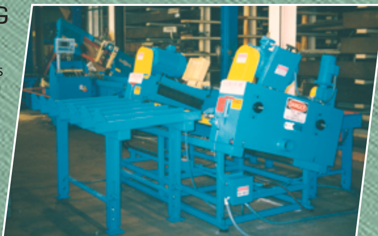
Automatic wire brush deburring machine integrated to a DoALL band saw. Cut parts are automatically rolled into the deburring unit, which then deburrs both ends simultaneously, ID and OD.
