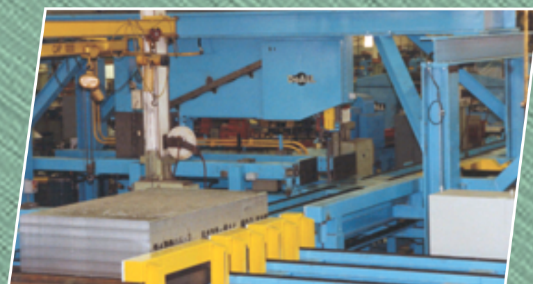
100 x 30 (2540 x 762mm) track-mounted band saw with heavy-duty material handling system for high-speed sawing of aluminum ingots features automated ingot handling and scrap removal.
