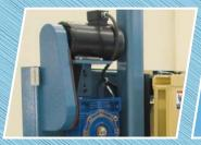
Powerful 5-hp (3.7kw) drive motor with AC inverter control for infinitely variable band speeds from 60 to 400 fpm (18 to 120mpm)
