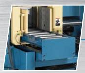
A floating style index vise pivots to accomodate crooked stock and increase accuracy. An underslung carriage and roller-style bed allow smooth, accurate material movement.
