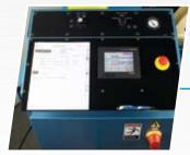
Control panel features a 6" TFT touch screen, mounted on a console with a built-in writing tray. Feed rate and feed force controls are also located on the console.
