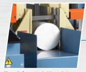
The split front vise holds workpieces on both sides of the blade to reduce burrs. A work height sensor detects material height to minimize head travel and reduce cycle times.
