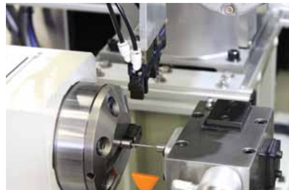
Robot gripper picks up completed part and loads the next one in a single operation.
