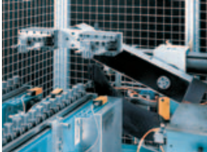
Just one example of many: two raw-parts are collected simultaneously from the workpiece magazine, ...
