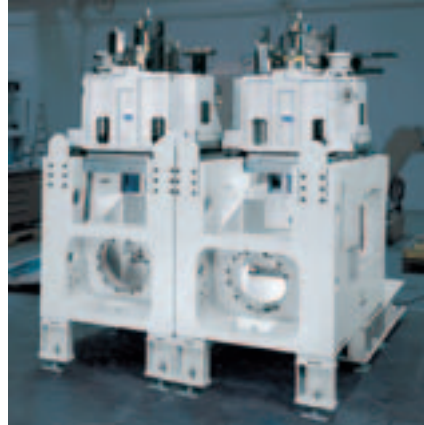
VSC 250 DUO: Separate, sturdy machine bases made of polymer concrete MINERALIT®. The two overhead slides are independently programmable
