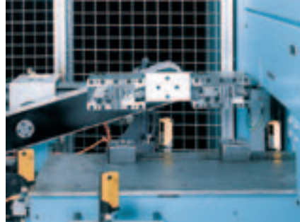
... deposited on the conveyor belt and transported to the pick-up position of the two spindles on the VSC 160 TWIN
