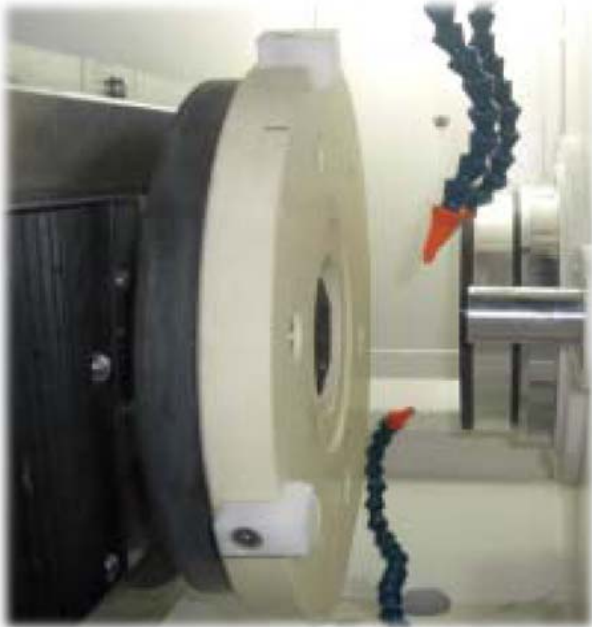
Showing actual work piece chuck (left) and grinding wheel (right, background) with two cooling fluid delivery nozzles.
