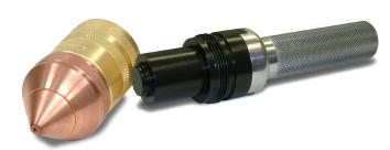
The special SpeedLoader fixture allows pre-assembly of the nozzle, nozzle retainer, diffuser, shield, and shield retainer. The operator can swap out pre-assembled consumable sets quickly and easily, minimizing down-time for consumable replacement or changeover. The SpeedLoader requires no expensive torch bodies and does not break any of the fluid connections when swapping parts - eliminating the risk of o-ring damage or leaks.
