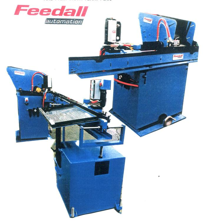
FEEDALL STANDARD MODEL 1700 D MAGAZINE TYPE SHAFT FEEDER. BAR/SHAFT DIAMETER RANGE 1/4 TO 1 1/4", AND LENGTHS FROM 3 1/2 TO 28". MODEL 1650 WITH 1" WIDE SILENT CHAIN, 72" LG. FEEDALL MODEL 1650 1 72 EXIT CONVEYOR WITH SHAFT KICK OFF BLOCK AND PART TRAY. DWG. PD 9122
