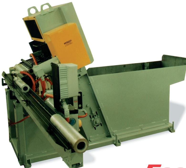
This Model 2220 was designed to feed heavy wall aluminum tubes 2" to 3" diameter by 12" to 20" long. The hopper was modified to accept loading bundles of tubes by a clam shell type gripper. The tubes are elevated from the hopper and discharged rolling to the rear into a magazine then escaped rolling one at a time to a rear mounted cross conveyor. The tubes are conveyed one at a time to a friction welder at a feed rate of 2 to 8 tubes per minute at a height of 42" above the floor.
