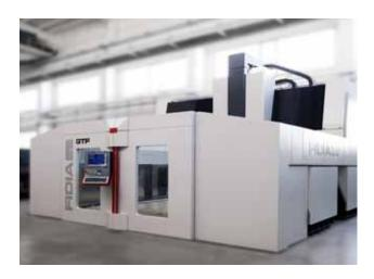
The axes cinematic chains may vary in order to achieve the highest working speed and acceleration. Rack & pinion tandem system drives X Y axis, while Z can be driven by ball-screw or rack & pinion, according to the stroke.
