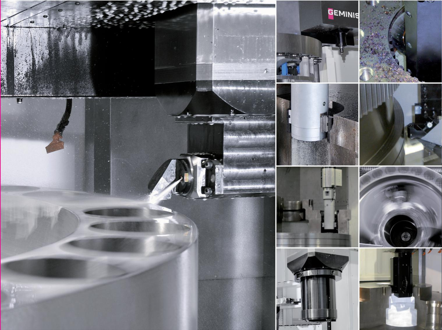
The versatility of the base machine of the GEMINIS VL range allows an approach to the complete machining of complex pieces. This approach is done by the integration of different accessories directly to the RAM through a coupling device specially developed by our team of engineers.
