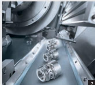
1: Integrated work piece removal comes as standard, work pieces up to: ø 50 × 150 mm / 2.5 kg (SPRINT 50), ø 65 × 200 mm / 4 kg (SPRINT 65) 2: Machined part conveyor is optional
