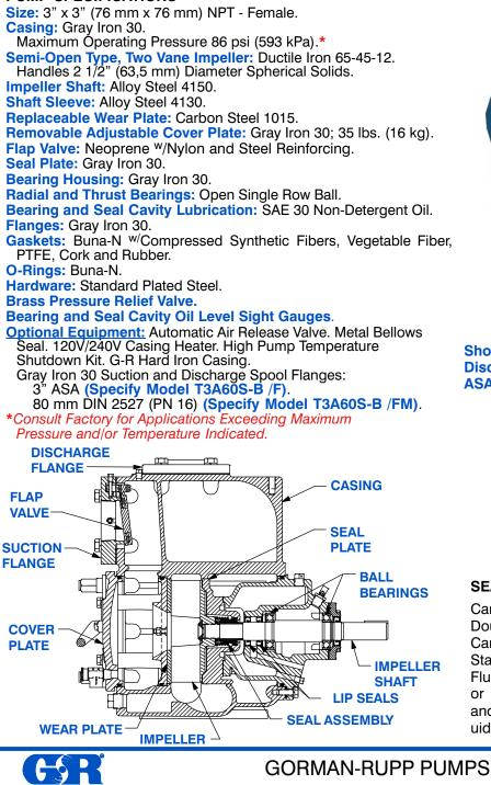
Shown with Optional Suction & Discharge Spool Flanges (Available in ASA or DIN Standard Sizes).
