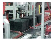
After the weight and jacket have been set, the ready molds are gently indexed forward to the pouring zone. At this point molds can be automatically indexed to pour from a single pouring station. Or, the pourer can move up the line to pour from multiple positions.
