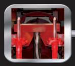
Detent cylinders, integrated into a rigid platen, lock the drag flask in alignment with the platen eliminating mold shift
