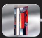
Zero clearance, Stainless Steel Linear Guiding System that precisely maintains positive alignment of the Cope and Drag molds throughout operations at the squeeze station.
