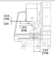
Distance from the spindle nose to the trunnion table pivot with maximum size part loaded while table is at +90° tilt
