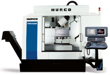
The VMX42SR was designed with a swivel head and horizontal rotary table to meet the demands of simultaneous 5-axis machining without monopolizing a large amount of floor space. With larger linear rails, bigger ballscrews, and heavier servo drives, the VMX42SR delivers superb surface finish and accuracy. The integrated Hurco control with WinMax\* software is full of powerful software features that increase productivity.
