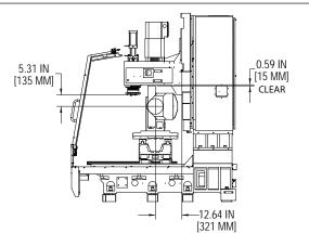
Distance from spindle nose to trunnion table pivot with maximum part with table at +90° tilt
