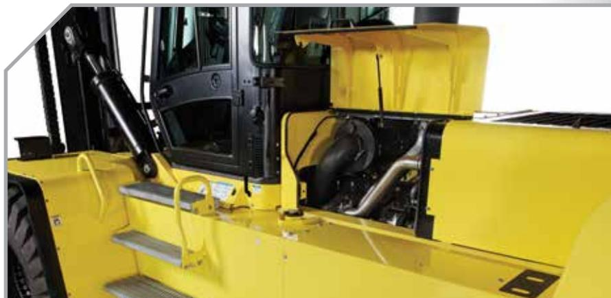
*Gull-wings provide easy access for quick service checks*
