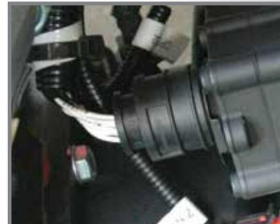
*Standard profile Deutsch pin connectors, IP64 compliant*
