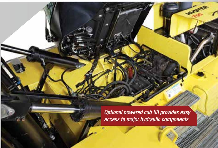
*Optional powered cab tilt provides easy access to major hydraulic components*
