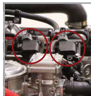
Coil over plug ignition design
