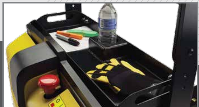
The W45Z HD with factory installed batteries includes an operator convenience tray with large storage area for stowing clipboards, pens, pencils and other items. Units equipped with a 9" battery box have several convenience tray options. (9" battery box option shown)
